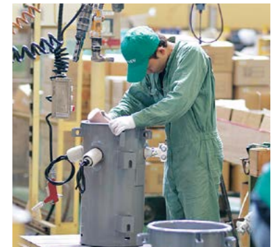
小形変圧器組立工程 Small transformer assembly process
