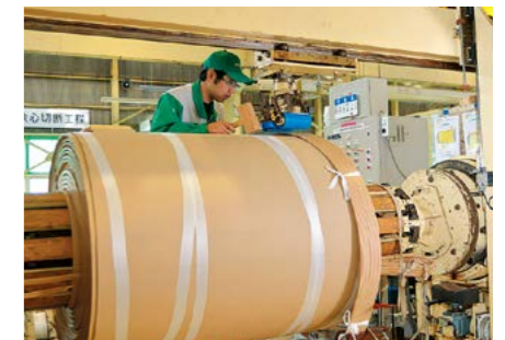
大形変圧器巻線工程 Large transformer coil winding process
