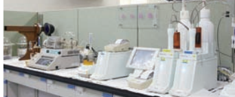
絶縁油特性試験 Characteristic tests of insulating oil
